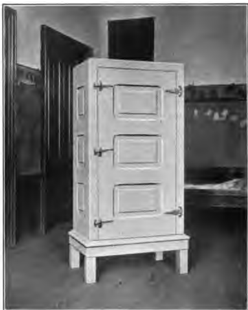
Disinfecting Cabinet Closed.
